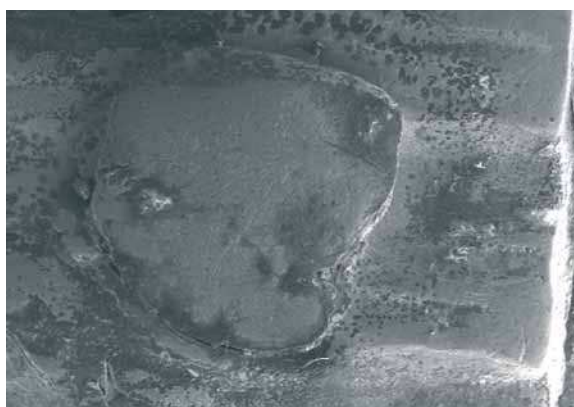
Fig.4.14. Loop with plain grooves (SHM 5814; SEM picture: Maria Wojnar-Johansson, AFL). Mag: 16X.
